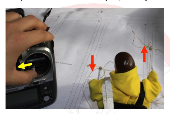
Moving the stick to the right moves the left arm up and the right one down, so that the wing turns right.
