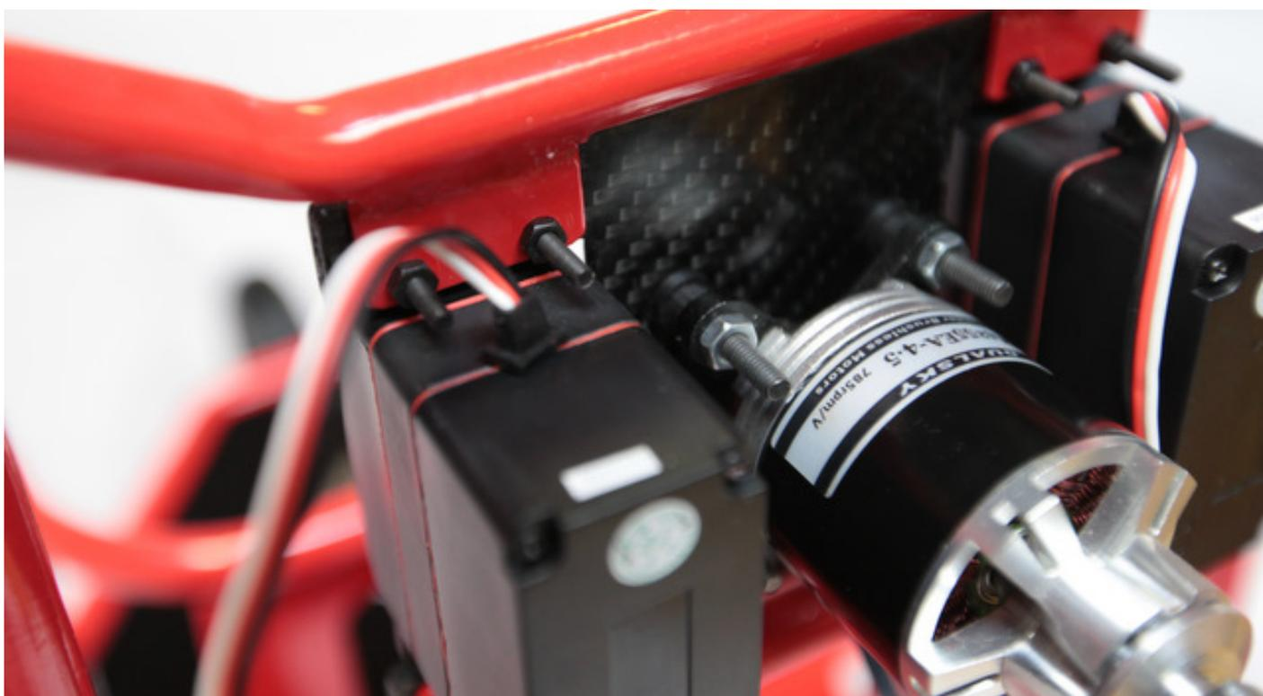
Screw the 8 nuts to hold the locking plate in position.
