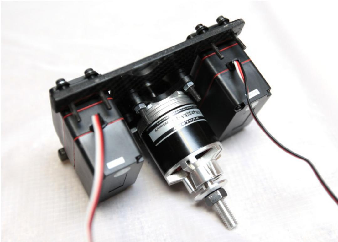
The 2 servomotors and the main motor are now installed, you can now secure them to the chassis.
