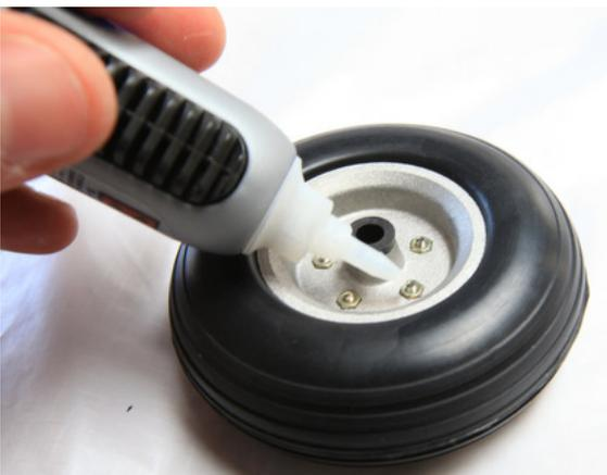
Secure the nuts using **thread sealant** or some **Loctite super glue**.
