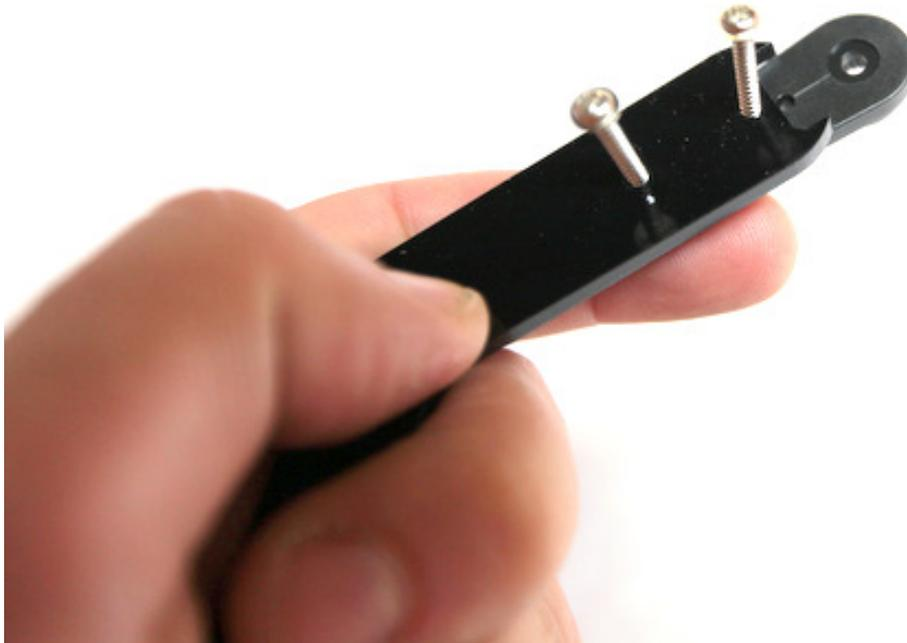
Cut the screw parts that are staying free on the other side of the plastic arms.
