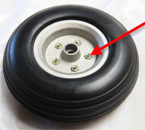
Insert the nuts on the other side of the rim. Screw the screws and the nuts firmly.
