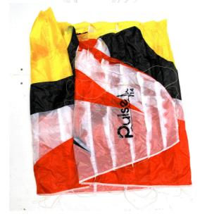
©Copyright by Opale-Paramodels 2013 FR Page **9** sur **12**  Finally put the risers back onto the wing and fold it 3 times in the other direction. The folding obtained should be about a hand wide so that it fits in its bag.
