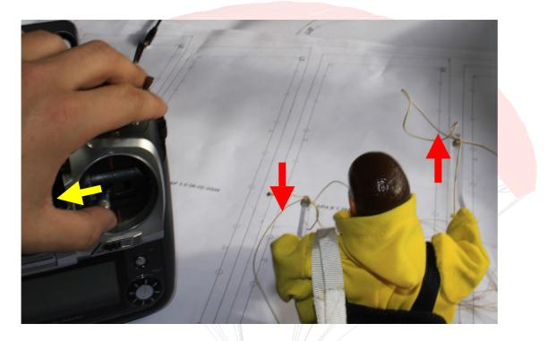
Moving the stick to the right moves the left arm up and the right one down, so that the wing turns right.
