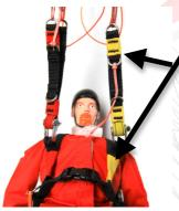
Fasten and secure the risers to the pilot as show on the picture above (Red risers to Red strap on the harness) If you pilot have the speedbar system, please refer to his manual for the settings
