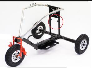
Install the platinum with the servomotors on the vertical holder by mean of 4x CHC M3-12 and 4x nut-lockings.
