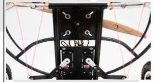
Aileron stick to the left, left servomotor go down in maximal low position.
