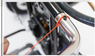
The brake bridle must slide in the ring fixed at the extremity of the arm.
