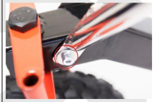
Tighten firmly the two screws located at the bottom of the holder.
