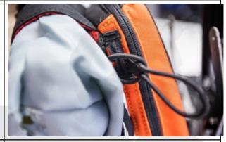
Fixe the elastic by making a full rotation around the shroud.
