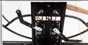
Aileron stick to the right, right servomotor goes down in maximal low position.
