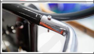
Then place a M3 nut, a M3 washer and a 2nd M3 nut to lock the whole thing.
