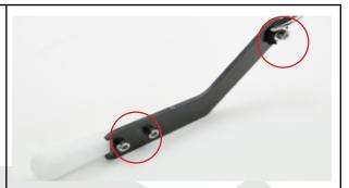
Power the two servomotors and position them into neutral position (signal 0). Then install the two rudder bars and put them horizontal.
