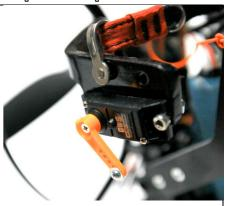
Max Speed position. The A lines are pulled down 10 to 20mm(depends on the wing you have)
