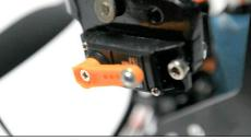
Take off position. The A lines are pulled down 5 to 10mm (depends on the wing you have)
