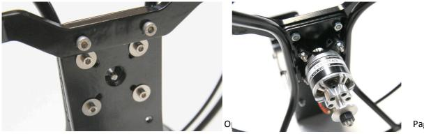
Then perform the installation of the propeller (Note that we recommend to use a propeller size which not exceeding 10inches. Besides, the ring can no longer do its aim). Do not forget to check the mounting direction of the propeller and the motor. The leading edge of the propeller should always be directed towards the front of the backpack.
