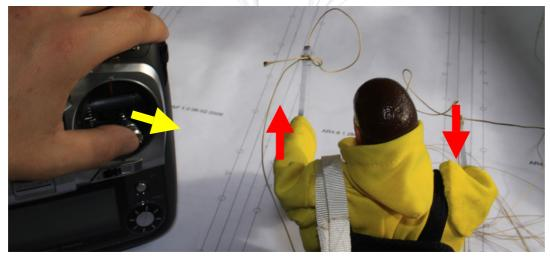
• Moving the stick down moves the arms down thus braking and slowing down the wing. Doing so allows you to reach the minimum speed before
