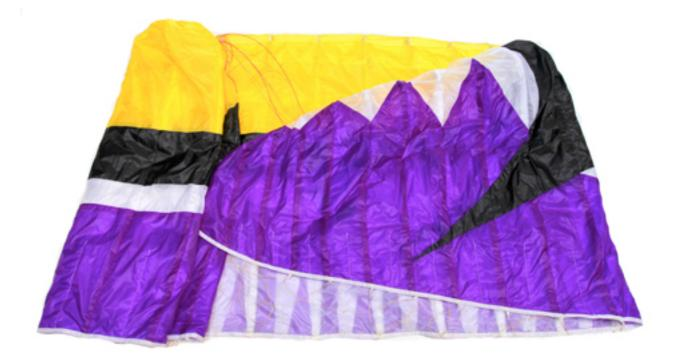
Finally put the risers back onto the wing and fold it 2 times in the other direction. The folding obtained should be about a hand wide so that it fits in its bag.
