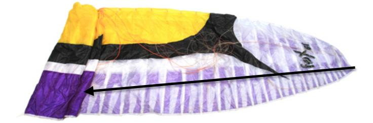
Pull both ends towards the wing center. Put the risers together at the centre to prevent them and the lines to get tangled up.
