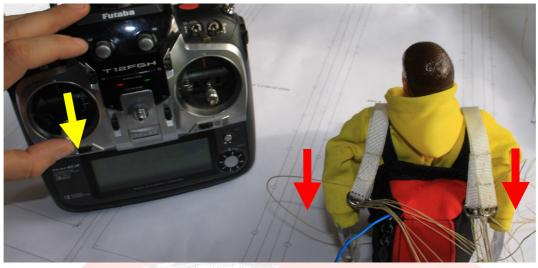
Moving the stick up moves the arms up thus accelerating the wing and so enabling it to reach its maximum speed.
