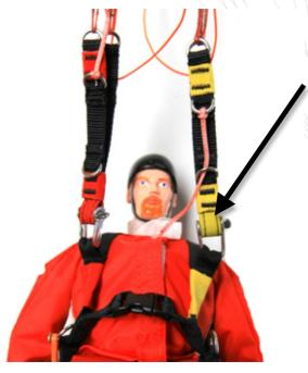
Fasten and secure the risers to the pilot as show on the picture above (Red risers to Red strap on the harness).
