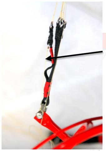
So, as it has just been mentionned, the way you will have to adjust the front lines closely depends on how much payload you are going to lift up in the air. When not loaded, the A lines should be 1 cm (0.39 in) lower than the B lines.
