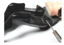
Enlarge the pre-drilled holes with a 2mm drill. (left photo)
