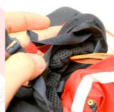
Be careful to highlight the servos gear of the Speed Bar System by the slot on the side of the harness. If you did not choose this option, please go to the next step.
