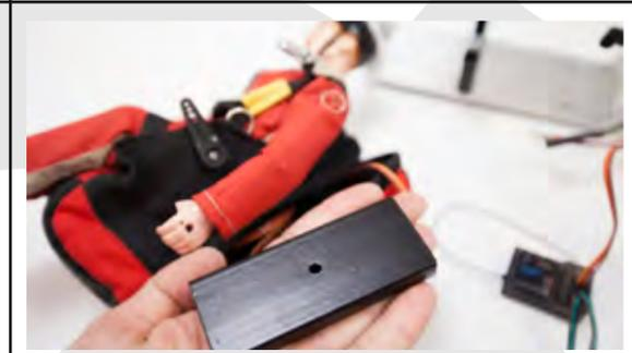
Insert the battery so the receiver and the mixer in the rear part of the harness. Close the whole.
