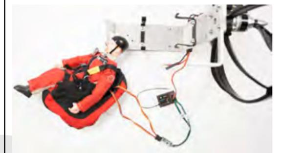
Install the ballast into your pilot, in fact of the harness (modulate the ballast quantity according to the wing size and the weather conditions of the day).
